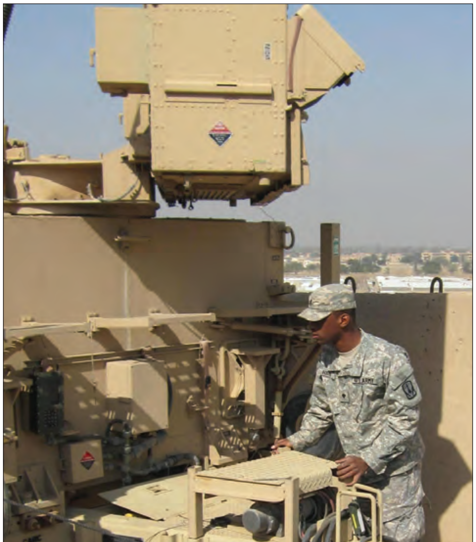
SPC Jermaine Foster, with Joint Task Force 5-5, conducts maintenance on the Sentinel Radar while at Victory Base, Iraq, last year. (Photo courtesy of 5th Battalion, 5th Air Defense Artillery Regiment)
