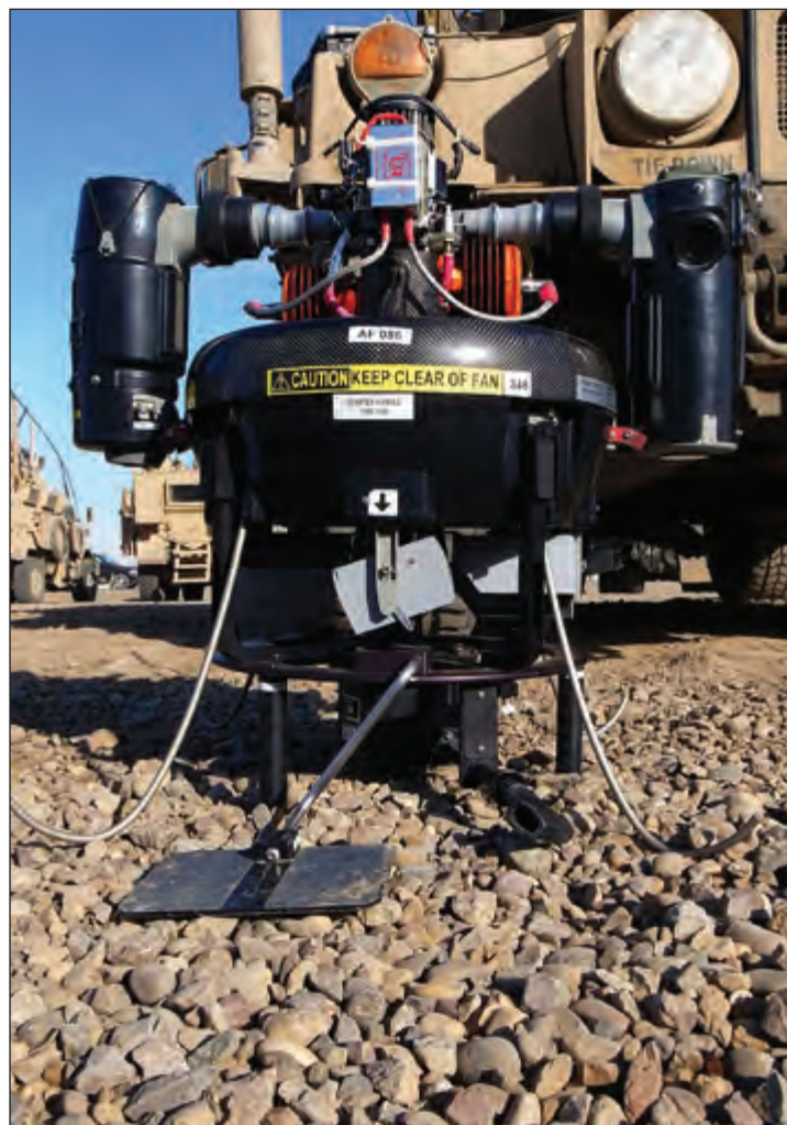
A gasoline-powered micro air vehicle, or gMAV, sits on display in front of a Humvee at the 4th Stryker Brigade Combat Team, 2nd Infantry Division headquarters at Camp Liberty. The gMAV is used by 38th Engineer Company during route clearance missions. (Photo by SGT Bryce Dubree, U.S. Army)
